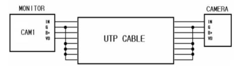
If you use UTP CABLE[CAT.5], Connect the rest 4 lines to GND after connecting 4 lines between monitor and camera.
